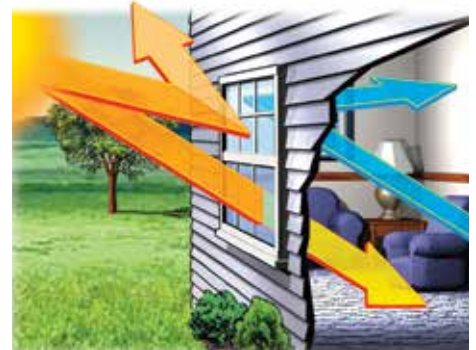
In summer months, Low-E glass helps block unwanted solar heat gain.
